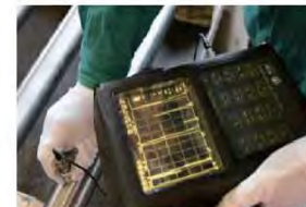
超声波无损探伤 Ultrasonic Nondestructive Testing
