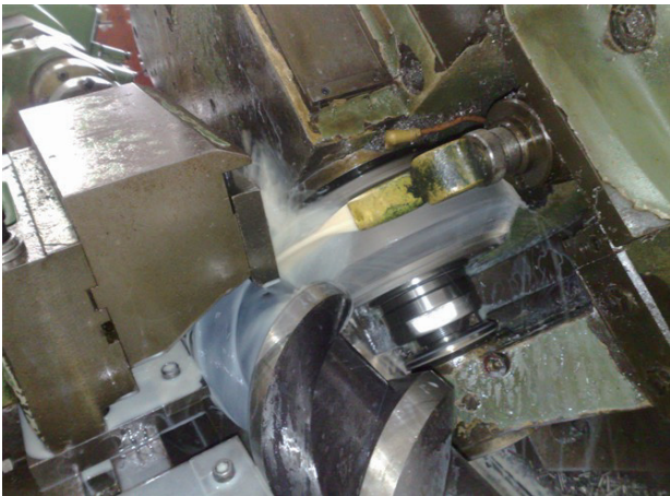
Milling Machine for Screw Pump Rotor
